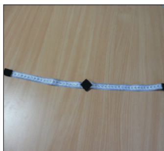
Image 2: The prototype occipital measuring device.
