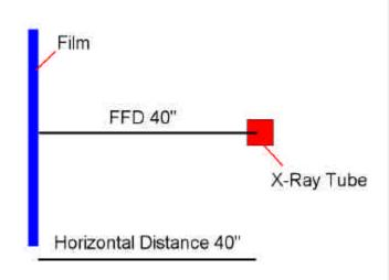
Here with no tube tilt the FFD and HORIZONTAL distances are the same.
