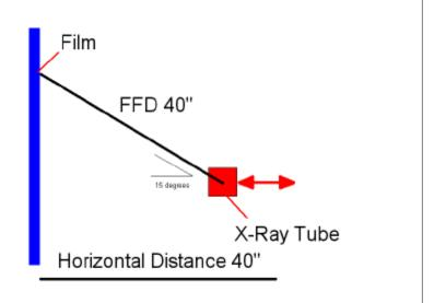
Here the HORIZONTAL distance has been reduced to compensate for the tube tilt.
